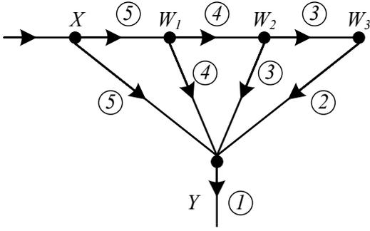
Fig. 4: DFG of a 4-tap FIR filter with signal transfer sequence. Step numbers are in circles.
