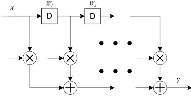
Fig. 1: Block diagram of a general FIR filter.
