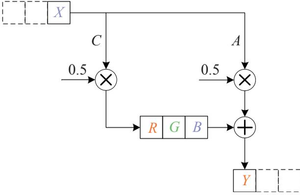
Fig. 3: Two-tap moving average filter in a three-phase configuration.
