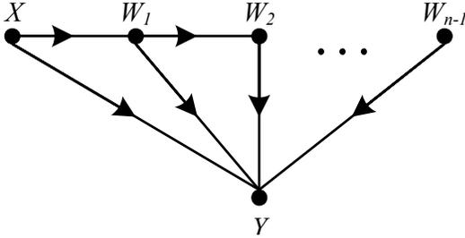
Fig. 2: DFG of an  $n$ -tap FIR filter.
