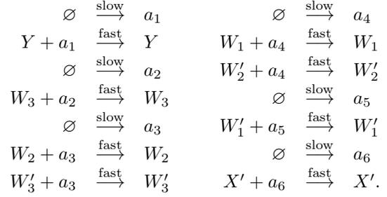
This example illustrates that the 4-tap FIR filter can be completed in 6 steps. In general, any  $n$ -tap FIR filter with all “1” coefficients can be completed by this assignment in  $n + 2$  steps.
